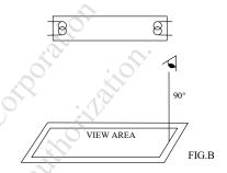
THE INSPECTION CRITERIA IS ACCORDING TO LINE OF SIGHT. INSPECTION SHALL BE MADE WITHIN THE HALF SECTION OF THE VIEWING CONE GENERATED BY LINE SEGMENT OF 45° WITH RESPECT TO THE VERTICAL AXIS FROM CENTER VERTEX OF LCD, THE FLUORESCENT LAMP AND THE CONE AXIS MUST BE PERPENDICULAR TO THE LCD SURFACE.
